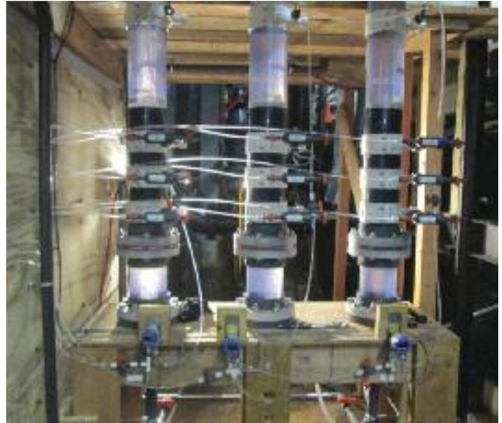
*Pilot test of manganese contactors*
